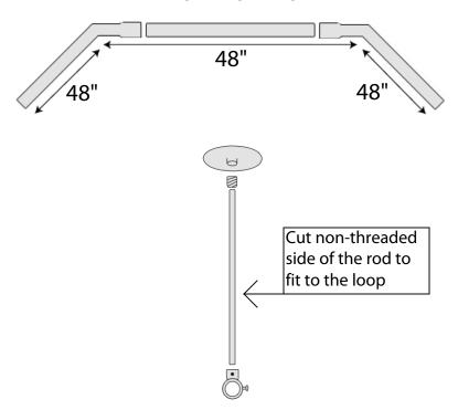
To shorten the neo-angle rod on any of the sides, cut at the three points shown on the instruction sheet.
