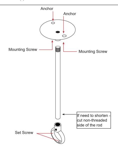
For extra strength, it is recommended to "drill and tap" set screws into both support and shower rod. Take set screws out and mark the location on the rods.
