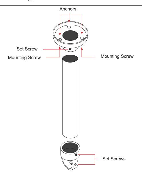
For extra strength, it is recommended to "drill and tap" set screws into both support and shower rod. Take set screws out and mark the location on the rods.
